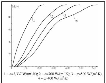
Fig. 2. Dependence of change in the mass flow M of the hydrogen desorbed from the metal hydride layer on the heat transfer factor
