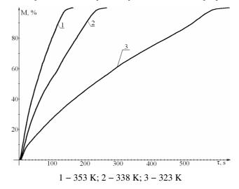
Fig. 3. Dependence of change in the mass flow M of the hydrogen desorbed from the metal hydride layer at  $\alpha=3,337$  W/( $m^2\cdot K$ ) from the coolant temperature
