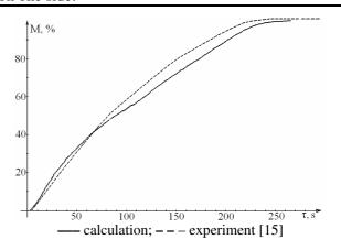
Fig. 1. Dependence of change in the mass flow M of the hydrogen desorbed from the metal hydride layer on the time  $\tau$
