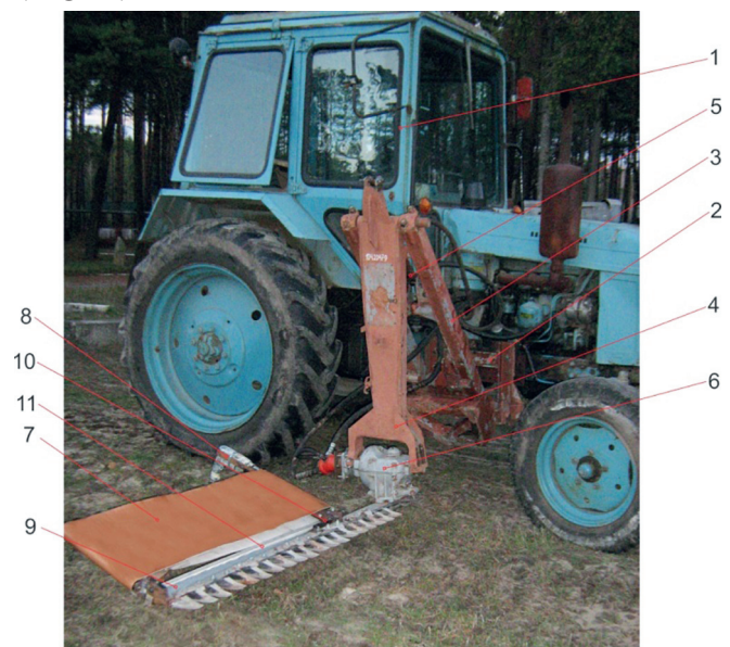
Fig. 1 – Model: 1- tractor MTZ-80, 2- binding frame, 3- arrow, 4- рукоять, 5- hydraulic cylinder, 6- the cutting device with the drive, 7- tor, 8- sorter drive, 9- drum contact device, 10- drum drive, 11- feeder
