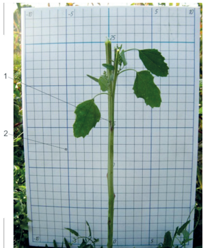
Fig. 2 – Determination of the acceleration of the apex of the cut stem of the plant: 1-stem of the plant; 2-sheet of paper with a grid
